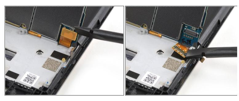
Use the edge of a spudger to pry up and disconnect the display flex cable from the motherboard.
