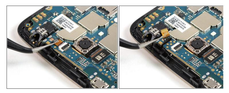
• Use a pair of tweezers to pull the flex cable out of the ZIF connector.
