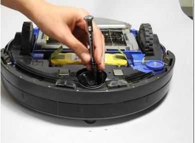
• Use Phillips #0 screwdriver to remove the two 9.64 mm screws.
