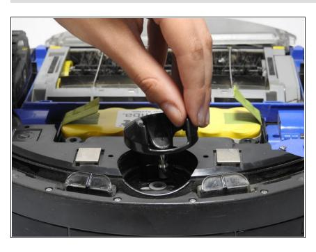
Pull out the castor wheel holder and remove it from the device.
