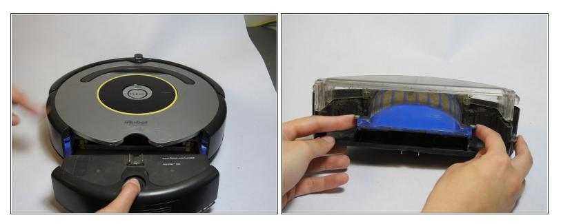
Gently pull out the cartridge. Then push in the yellow tabs to remove the filter.
