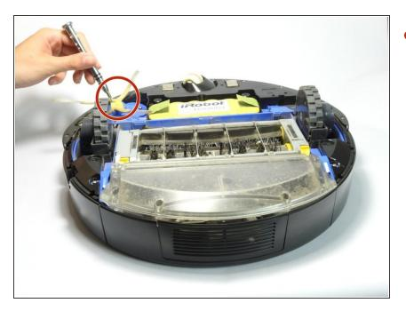
Remove the single 6.1mm Phillips#0 screw from the side brush.
