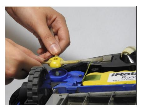
• Lift the side brush, removing it from the motor.
