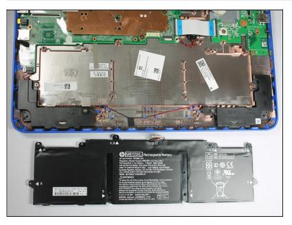
Remove Battery Assembly from device.
