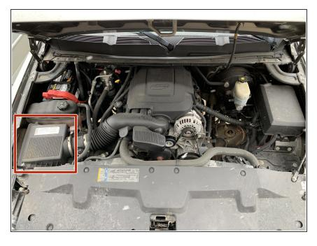
The airbox is located in the front left corner of the engine bay.
