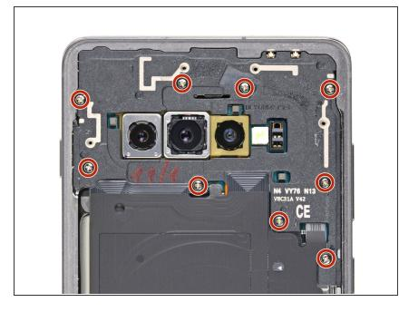
Remove the nine 4 mm Phillips screws securing the top midframe to the phone.
