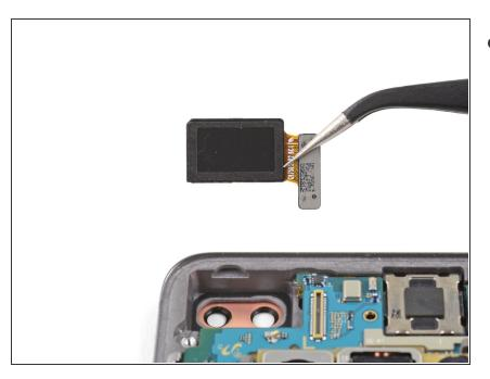
Remove the front-facing camera module.
