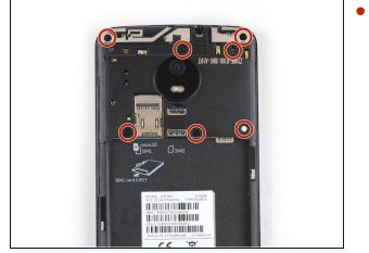
Remove the seven 3.3 mm Phillips #00 screws.
