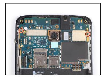
Remove the two 2.9 mm long Phillips #00 screws securing the motherboard.
