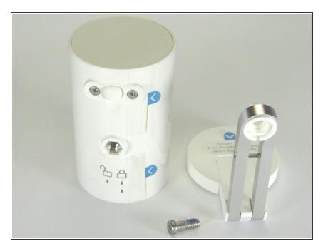
Remove the screw holding the mounting bracket to the ring camera with a Torx T15 Tool.
