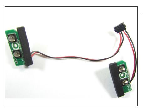
Close up view of the IR Light LEDs
