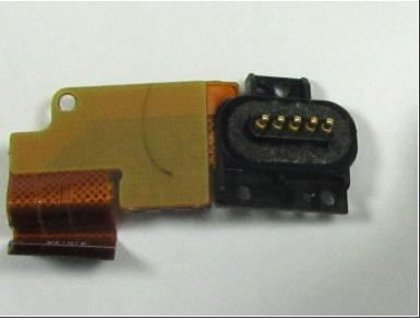
Once the battery holder compartment has been separated from the ring camera enclosure, the battery interface PCB can be pried off the battery holder compartment using the Spudger Tool.
