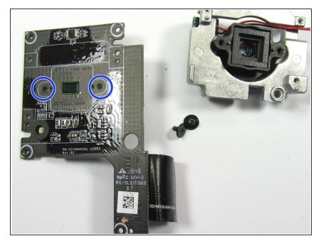
To separate the camera Lens from the Camera Sensor PCB, remove the two PH00 screws from the back of the PCB.
