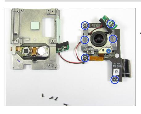
To separate camera, and IR Light LEDs, from camera body remove the six PH00 headed screws.
