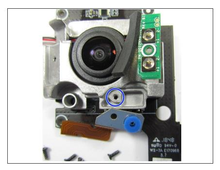
To remove the MEMS Microphone, remove the PH00 screw.
