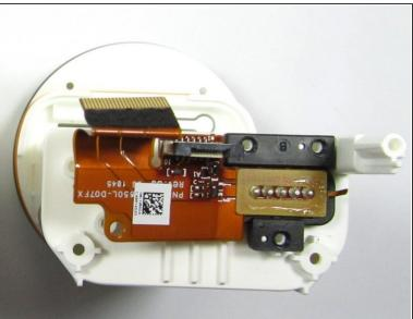
• With Spudger Tool, gently press down on the Battery Holder from the topside until it become loose. The Battery Holder, at this step, is held in place via an O-Ring. Once the Battery Holder becomes loose, gently pull it out the rest of way via the bottom of the ring camera enclosure.
