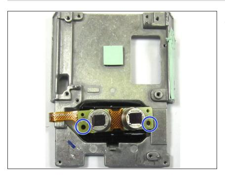
To remove the PIR Sensors, remove the two PH00 screws holding the PIR Sensor board to the Camera Body.
