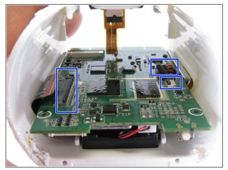
Loosen the two flex cables by using the Spudger Tool to pry up the flex connector tension strip. Then use the Spudger Tool to pry up the fourwire connector cable. This cable will pop up from the connector
