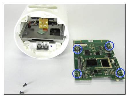
Remove the four PH00 screws holding the PCB in place. Then use the Spudger Tool to gently pry the PCB from the double stick tape holding the PCB.
