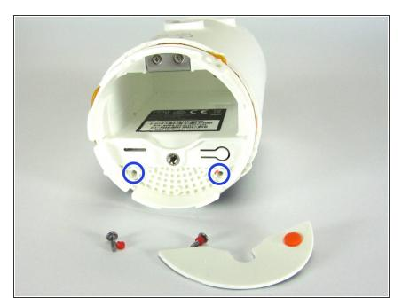
Remove rubber pad in the battery cover with the Spudger Tool or flat head screwdriver to reveal PH00 screws that hold the battery compartment to the ring camera enclosure. Remove the PH00 screws.
