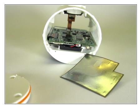
• Remove the RF Shield with the Spudger Tool. This can be removed during this step or after the PCB has been removed from the ring camera enclosure. Removing the RF Shield now helps simplify additional steps that may be needed in the teardown.
