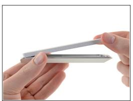
To open the enclosure, pull the top half down toward the wedged end and lift it away from the bottom half.
