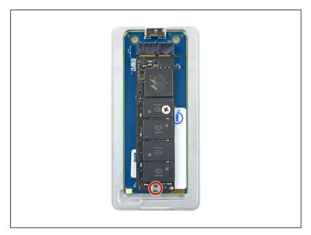
Use a T5 Torx driver to install the 6.5 mm screw securing the bottom of the SSD.
