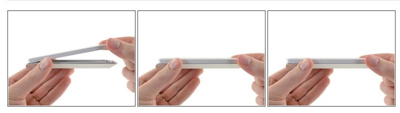
Reinstall the top half of the enclosure and slide it closed.
