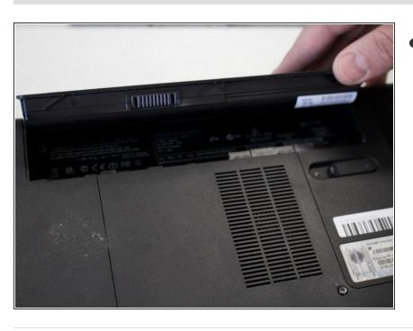
Lift and remove the battery from its compartment.
