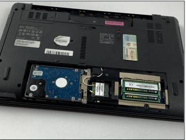
Using a plastic opening tool, lift up the panel and remove it completely.
