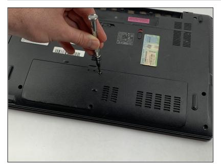
Unscrew the 8.6 mm screws on the back panel with a Phillips #0 screwdriver.
