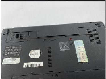
• Pull the other switch completely while the red unlock symbol is still present. The battery pack should pop up a bit.
