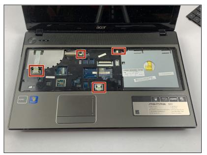
• Locate the 4 connectors that must also be disconnected.
