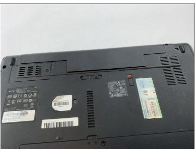
Pull the other switch completely while the red unlock symbol is still present. The battery pack should pop up a bit.
