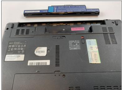
Remove the battery pack via the indentation at the top of the battery in between the two switches.
