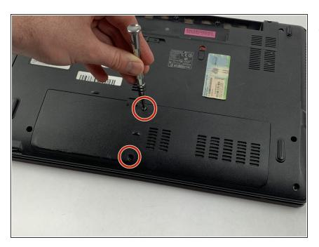
Unscrew the two 8.6 mm screws using a Phillips #0 screwdriver.
