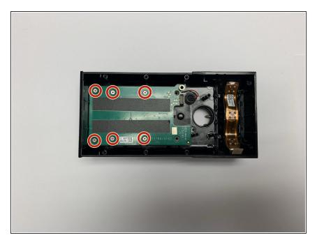
Remove the six silver 4.5mm Phillips #00 screws holding the daughterboard into the device.
