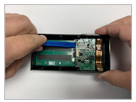
Carefully disconnect the camera board from the daughterboard by sliding a plastic opening tool between the camera board and the daughterboard.
