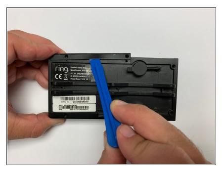
Pry off the aluminum plate using a plastic opening tool.
