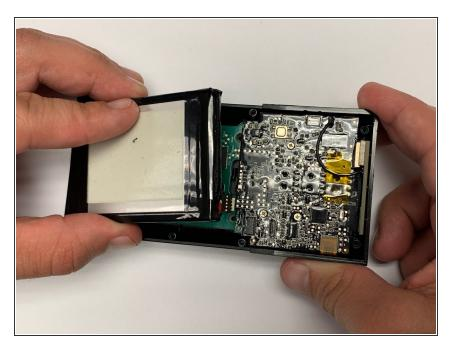
Use a plastic opening tool to loosen the adhesive holding the battery in place and remove the battery by hand.
