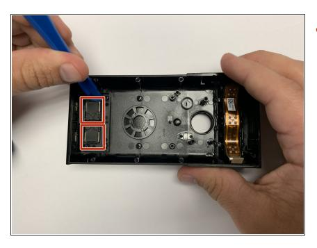
Using a plastic opening tool, remove both of the speakers.
