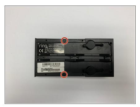
Remove the two 6mm Phillips #00 screws that were under the aluminum plate.
