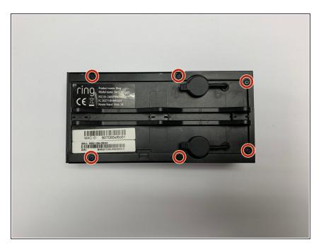
Remove the six 6mm Phillips #00 screws from the back of the device.
