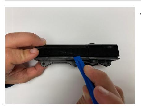
Pry off the back cover using a plastic opening tool.
