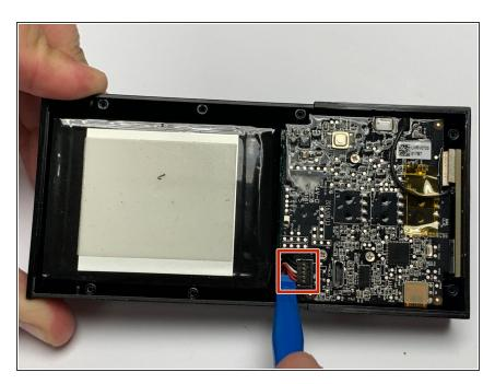
Disconnect the battery power leads using a plastic opening tool.
