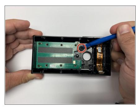
Use a plastic opening tool to carefully pry the microphone from the housing.
