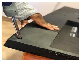
Carefully unscrew all of the screws in the back of the TV.
