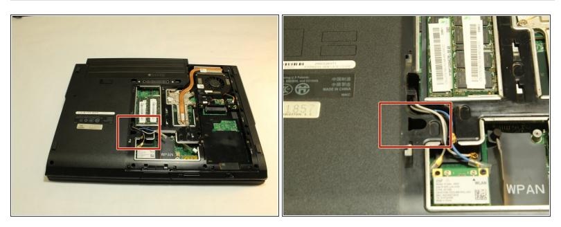
• Locate the slot for the CD ROM ejector found inside the red box shown.
