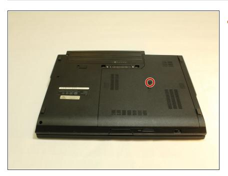
• Remove the screw located in the red circle shown.
