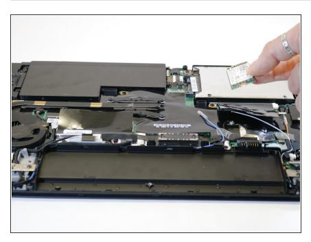
Pull the network adapter out of the device.
