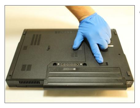
Locate the battery's release switch and slide it to the right
