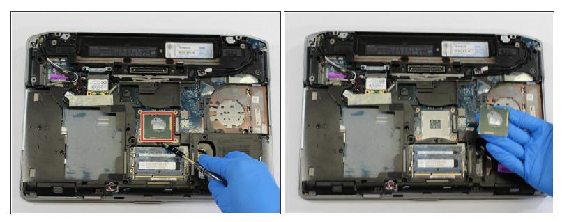
• Lift the CPU out of the motherboard assembly.
