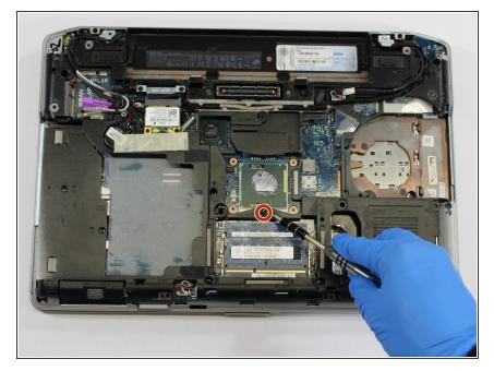
Use the flat end of a spudger to rotate the lock 180 degrees counterclockwise to unlock the CPU.
