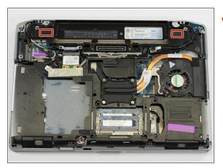
Remove the battery by pushing the tabs outward, then removing the battery from the device.
