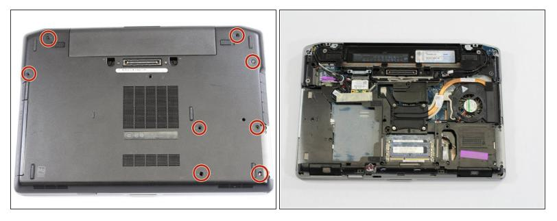
Remove the eight screws holding down the rear panel using a Phillips #0 Screwdriver. Carefully remove base cover by hand.
