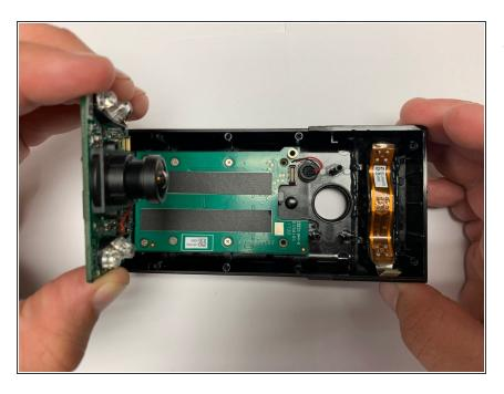
Lift the camera board out of the housing using your hand.
