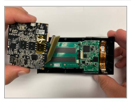
Remove the motherboard from the device by hand.
