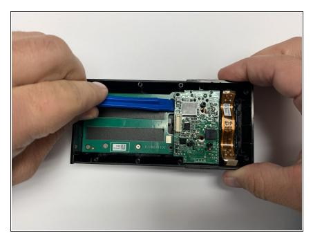
Carefully disconnect the camera board from the daughterboard by sliding a plastic opening tool between the camera board and the daughterboard.
