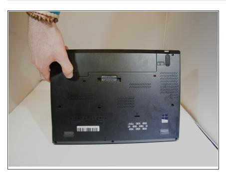
Slide lock button 1 to the unlock position and gently slide away from your body.
