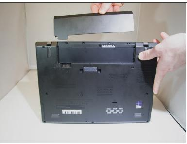
Slide lock button 2 to the unlock position and continue gently sliding until the battery is removed.
