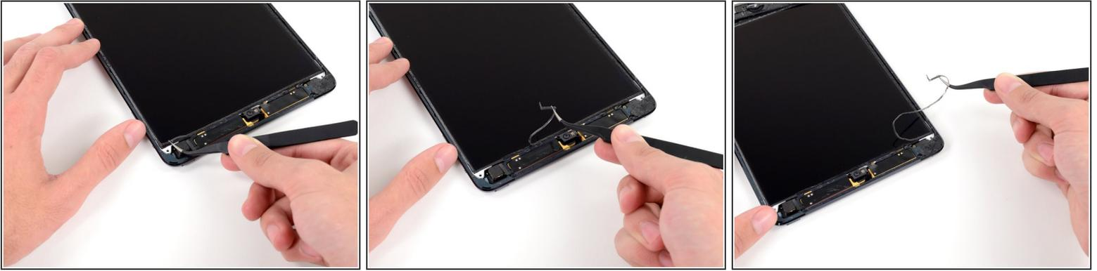
**i** A thin strip of foam tape on the LCD frame is covering a piece of tape connecting the LCD to the panel beneath it. To proceed, you'll have to break and peel up some of the foam tape to expose the tape hidden beneath.
