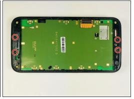
With a T4 screwdriver, remove the 10 "yellow" 2mm screws and 4 "black" 2mm screws.
