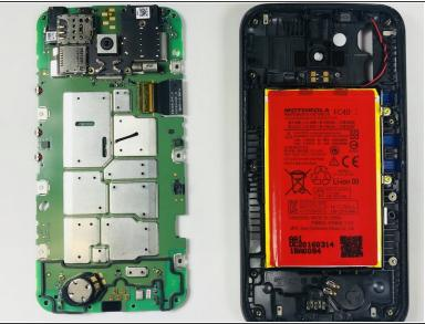
Use the metal spudger and lift the back cover on the bottom side of the phone (this is attached to the motherboard).
