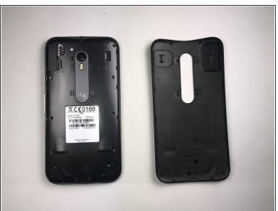
Use the plastic opening tool to open the back cover as shown in the photo.
