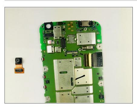
Remove the front camera from the device.
