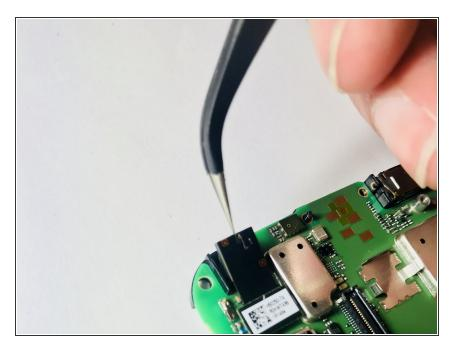
Using tweezers, pry open the black front camera cover and remove it from the motherboard.
