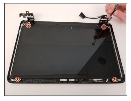
Remove the four 3-mm JIS #0 screws.
