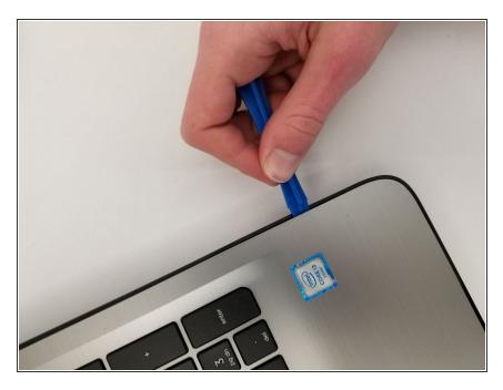
Unclip the keyboard surface from the base using an iFixit opening tool around the entire border.
