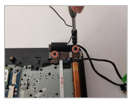
Remove the two 6.5-mm screws from the fan side of the computer.
