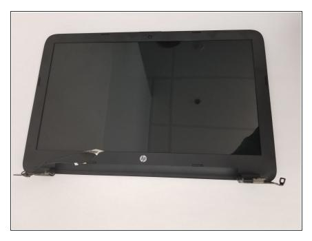
Lay the display with its back on a flat surface.
