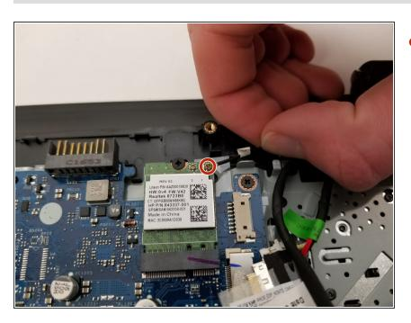
Unplug the wire attached to the wireless adapter.
