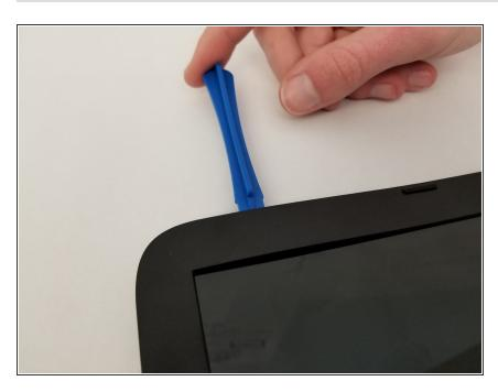
Pry open the screen cover using an iFixit opening tool around the entire screen.
