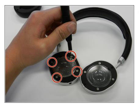
Remove the four 5mm screws from the earpiece with a Y1 Triwing screwdriver.
