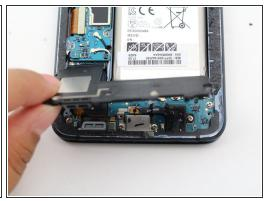
Remove the loudspeaker assembly using the flat end of a spudger.
