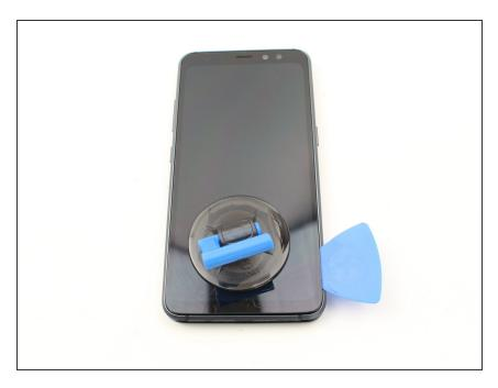
Insert an opening pick into the gap between the display and the frame created by pulling up on the suction cup.
