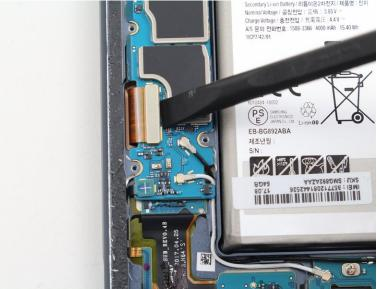
• Disconnect the display flex cable on the motherboard using the flat end of a spudger.
