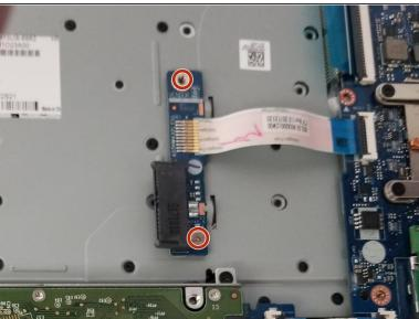
Unscrew the two 3mm JIS #0 screws that hold the optical drive (CD-reader) connection to the device.
