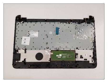
Make sure there is nothing else attached to the keyboard cover so all that remains is the keyboard and touch-pad.
