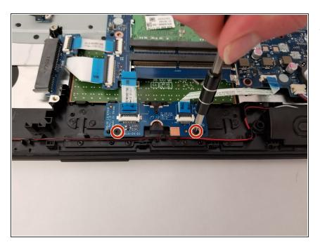
Remove the two 3mm JIS #0 screws that secure the touchpad board.
