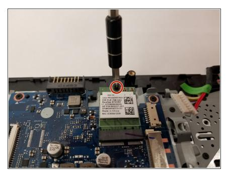
Remove the single screw from the wireless card and gently remove the drive.
