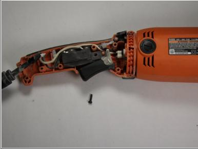
Remove the one M4 x 14 mm screw using a Phillips screwdriver.
