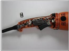
• Using a hex head screwdriver, remove the two 8-16 x 1/2in screws.
