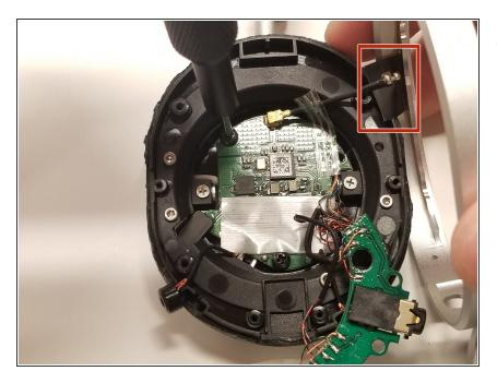
• Pull the black tape holding the connector in place.
