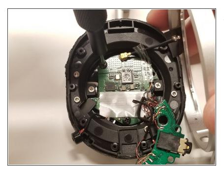
• Solder the new Bluetooth connector into place.
