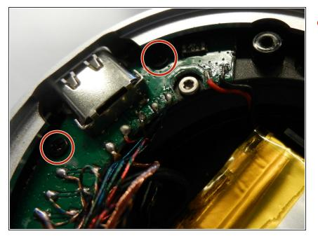
Remove the two 2mm screws shown with a JIS #00 screwdriver.
