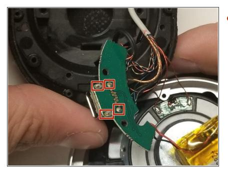
Lift up the mother board with the attached charging port to see the soldering points. You must desolder these points in order to detach (and re-attach) the charging port.
