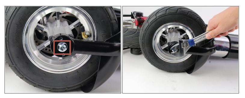
Using an adjustable spanner wrench, rotate the 165 mm bolt counter-clockwise to remove.
