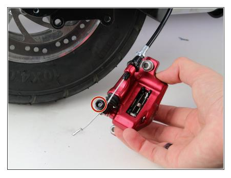
Remove the one, 14 mm Hex #4 screw pushing down the brake wire to the brake mechanism on the bottom.
