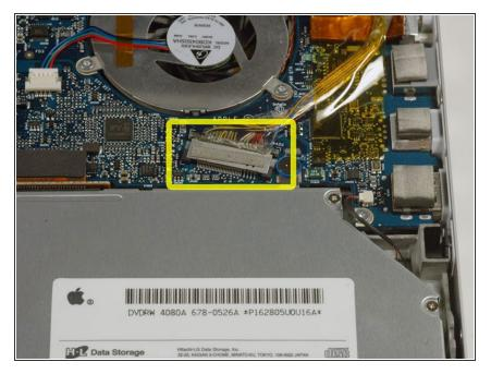
Disconnect the display data cable from the logic board.
