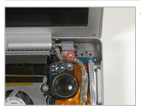
Remove the silver T6 Torx screw securing the ground loop on the display data cable to the casing.
