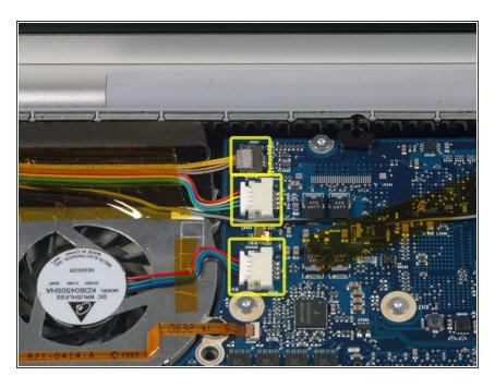
Disconnect the iSight, inverter, and left fan cables from the logic board by gently pulling in the direction of each cable.
