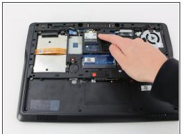
Slide the base cover down slightly and remove it to find the WLAN card.
