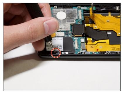
• Take out the one 3mm screw on the motherboard with the Phillips #00 screwdriver.
