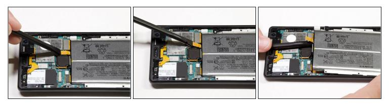
• Use the spudger to pry up the battery flex connector to pop the battery out.
