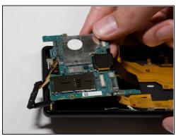
• Use the spudger to lift the motherboard out of the phone.
