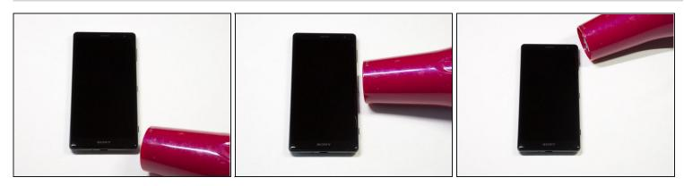
Weaken the glue that is keeping the screen in place by heating up the edges of the phone with a hair dryer or heat gun.
