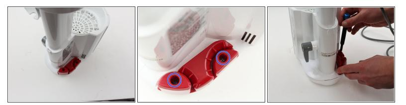
• Remove the two 19mm Phillips #2 screws located in the red plastic piece behind the filter.
