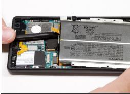
• Use the spudger to pry up the battery flex connector to pop the battery out.
