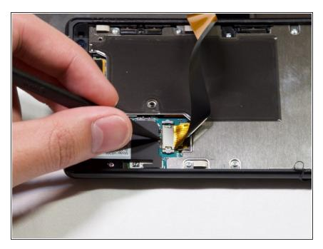
Gently remove the connector by using a spudger to pop it off.
