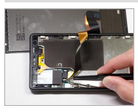
Remove the bracket covering the connector by grabbing one side of the bracket with angled tweezers and gently pulling it off.
