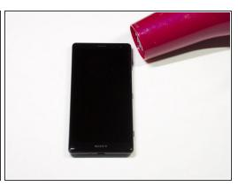
Weaken the glue that is keeping the screen in place by heating up the edges of the phone with a hair dryer or heat gun.
