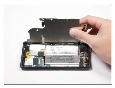
Lift the metal screen shield out of the phone.
