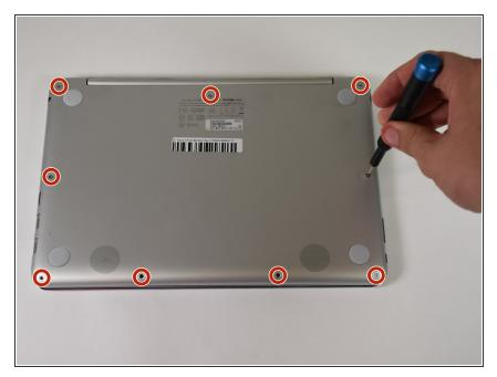
Use the T5 screwdriver to remove the nine 2.1 mm screws from the bottom of the device.
