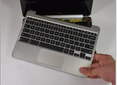
Grip the keyboard and carefully pull it off the device.
