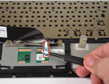
• On the back of the keyboard assembly, use the tweezers to pull the white cable from the track pad.
