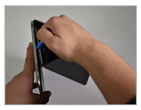
Use the iFixit opening tool to remove the back of the laptop.
