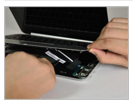
Use the blunt nose tweezers to separate the keyboard from the internal components.
