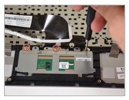
Remove the three 1 mm screws from the track pad using the JIS 00 screwdriver.
