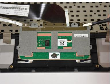
Grip the track pad with the tweezers and slide it up and out of the keyboard assembly.
