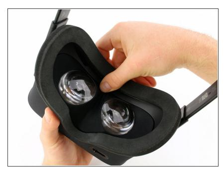
Pull firmly from the top of the headset facial interface to remove the foam frame.
