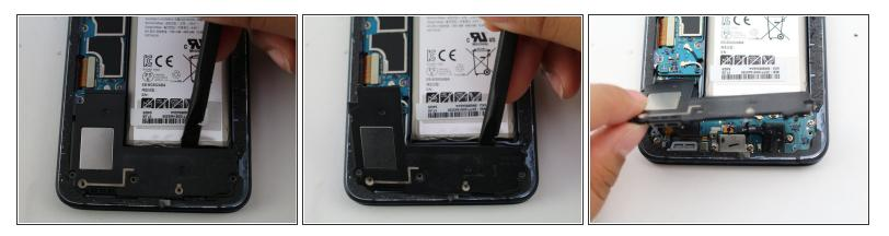
• Remove the loudspeaker assembly using the flat end of a spudger.
