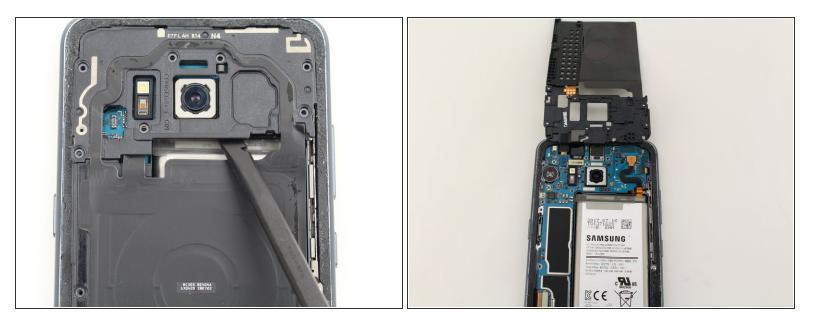
• Remove the NFC antenna and charging coil assembly using the flat end of a spudger.
