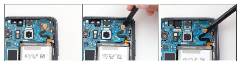
• Disconnect the battery flex cable using the flat end of a spudger.
