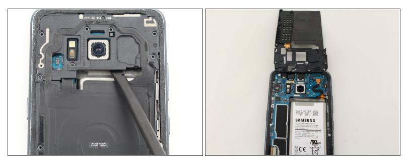
• Remove the NFC antenna and charging coil assembly using the flat end of a spudger.
