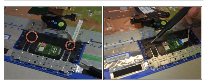
Remove the two 2mm #000 Phillips screws.
