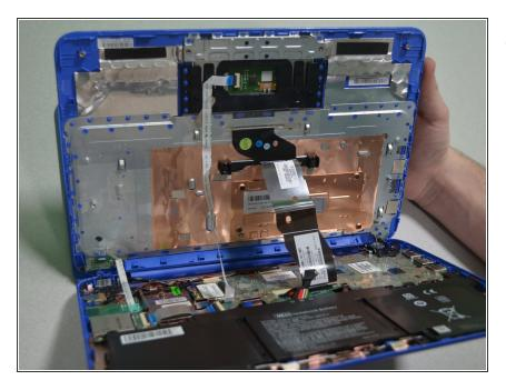
Lift the keyboard out of the laptop to remove it from the device.
