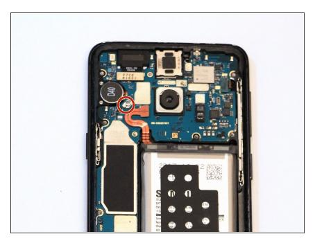
Remove one 3mm screw with a #000 Phillips screwdriver.
