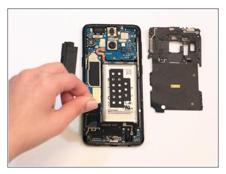
Remove the speaker cover/antenna assembly.
