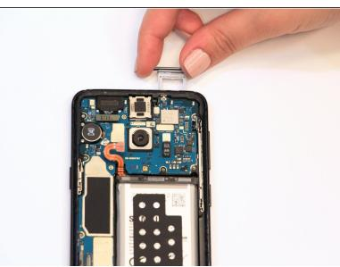
Take out the SIM card by using a SIM card remover or unbent paper clip to depress the release lever.
