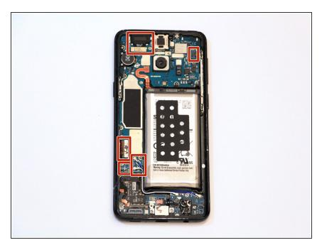
Disconnect 6 cables by prying apart the connections with a spudger.
