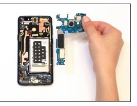
• Remove the motherboard by prying it out with the spudger.
