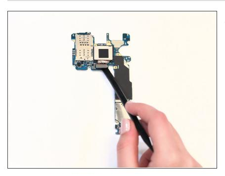
Disconnect one connector by prying it apart with the spudger.
