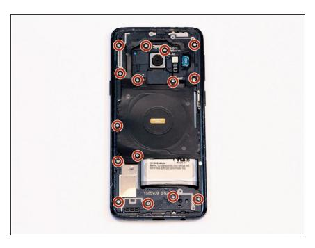
Remove fifteen 4mm screws with a #000 Phillips screwdriver.
