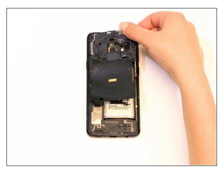
Remove the NFC coil assembly.
