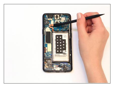
Disconnect the battery by using a spudger to pry open the connection.
