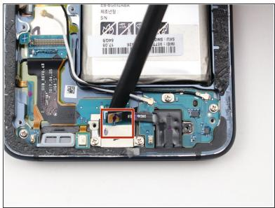
Disconnect the headphone jack flex cable using the flat end of a spudger.
