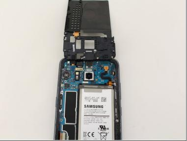
Remove the NFC antenna and charging coil assembly using the flat end of a spudger.
