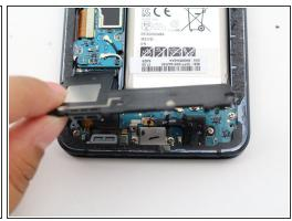
Remove the loudspeaker assembly using the flat end of a spudger.
