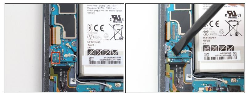
Disconnect the charging port flex cable using the flat end of a spudger.
