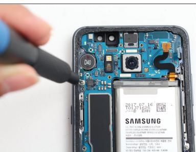
Remove one 3.5 mm screw using a Phillips #00 Screwdriver.
