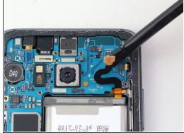
Disconnect the battery flex cable using the flat end of a spudger.
