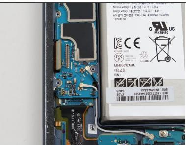
The motherboard rests on top of the daughterboard, and there is a flex cable connecting them. Disconnect the flex cable that connects the motherboard to the daughterboard using the flat end of a spudger.
