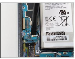
Disconnect the black and white antenna cables using the flat end of a spudger.
