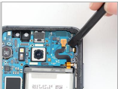
Disconnect the Volume Up, Volume Down, and Bixby button flex cable using the flat end of a spudger.
