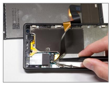
Remove the bracket covering the connector by grabbing one side of the bracket with angled tweezers and gently pulling it off.
