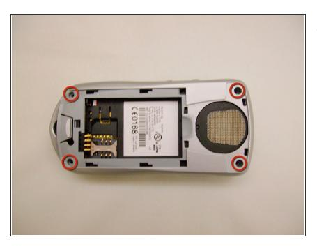
Remove the four screws indicated in the picture with a #T6 Torx Bit screwdriver and set them aside.
