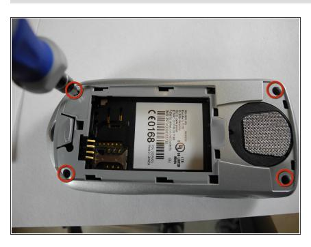
Screw and tighten the four screws on the back side of the phone.
