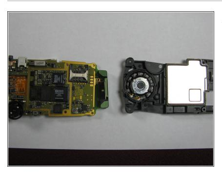
The black battery casing and logic board can now be separated for the following steps.
