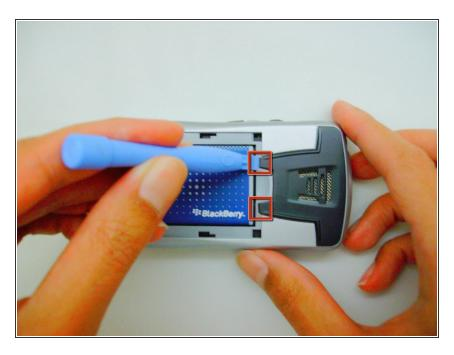
Use a plastic opening tool or fingernails to unclip the two hinges of the speaker covering and remove it.
