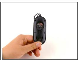
Remove the back panel by firmly sliding it towards the strap.
