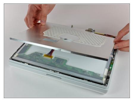
• Carefully remove the thin steel LCD cover.
