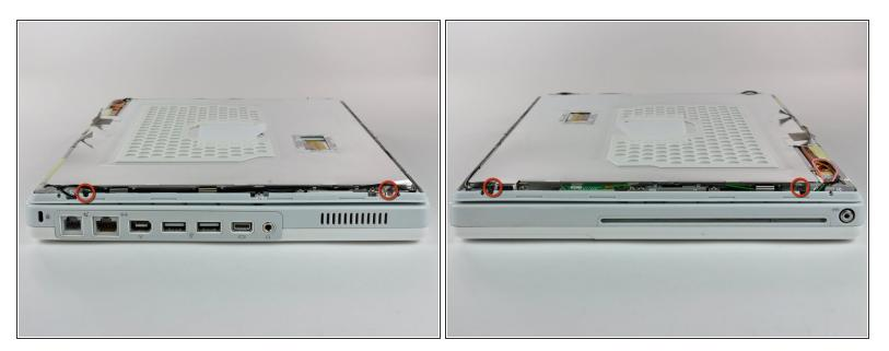
Remove the two Phillips screws securing the left and right sides of the LCD to the frame of the clutch hinges (four screws total).
